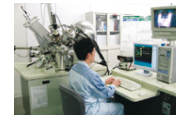
Using X-ray photoelectron spectroscopy to analysis fine matter adhered to a machined surface
