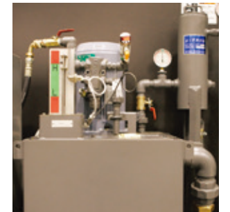
Spindle-through coolant 3MPa
