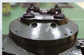
Taper-type pallet clamping mechanism
