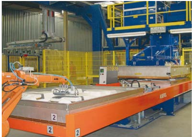
Turntable machine with feed robot for the welding of reinforced sections onto floor carpets.
