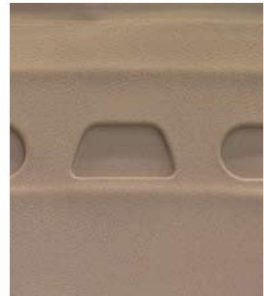
Slush-moulded skin in the galvano (tool)
