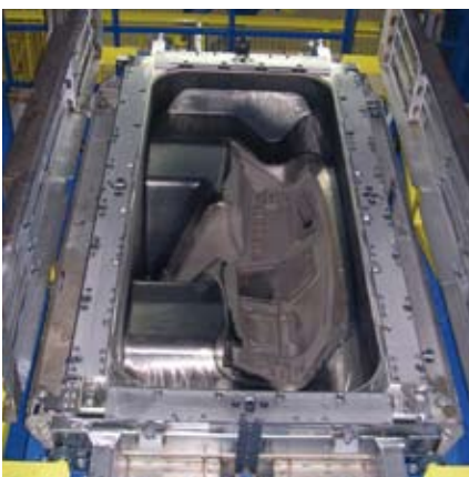
Galvano in IR-preheating station
