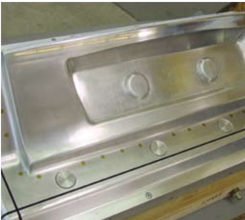
Highly-polished vacuum-capable forming tool.
