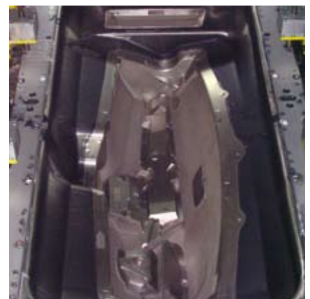
Galvano with slush-moulded skin at the removal station
