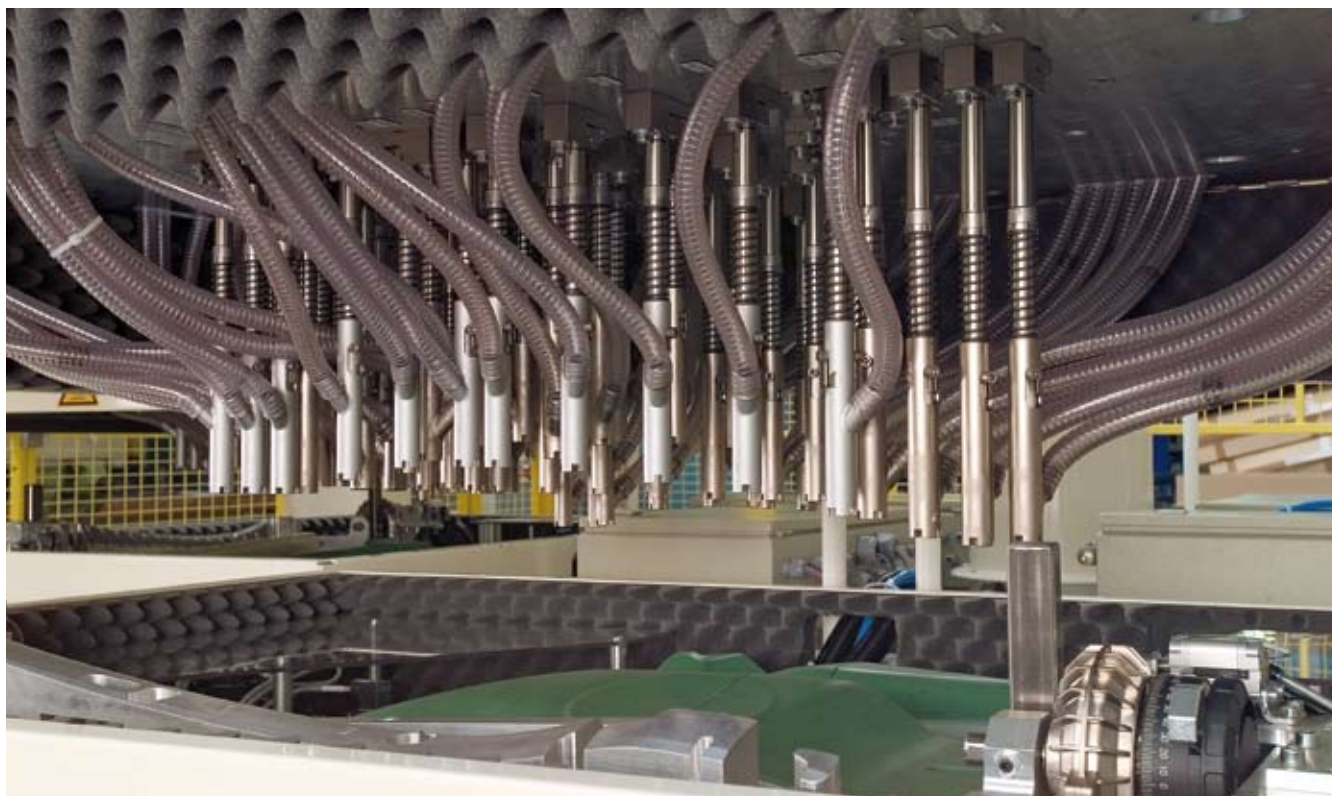
Riveting of a complete door lining using the ASC riveting system.
