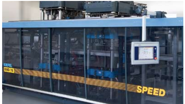
Series KMD machine for forming the decorative trim elements.
