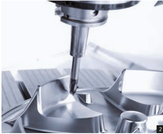
1: 5-axis simultaneous machining 2: 18,000 rpm motor spindle 3: Linear drives and measuring systems in all axes
