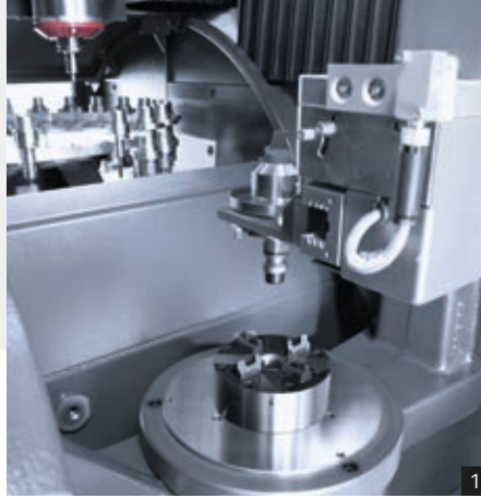
1: Stable pallet change of < 30 seconds
