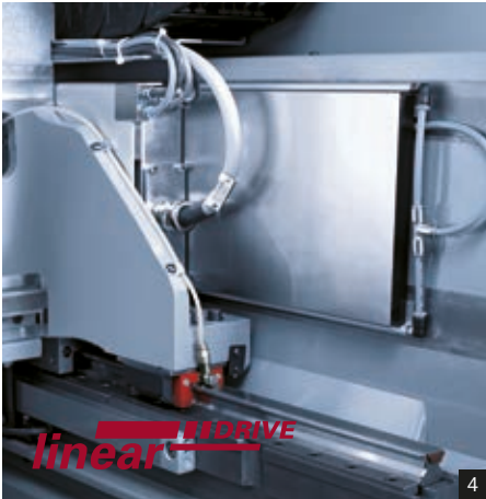
1: Workspace – integrated NC swivelling rotary table 2: 5-axis complete machining of a bone plate in titanium 3: Finish machining of a CoCr femur component 4: Linear drive in X / Y / Z with > 2g 5: 24-pocket tool changer as standard (optional: 60 pockets) 6: Watch mechanism plate
