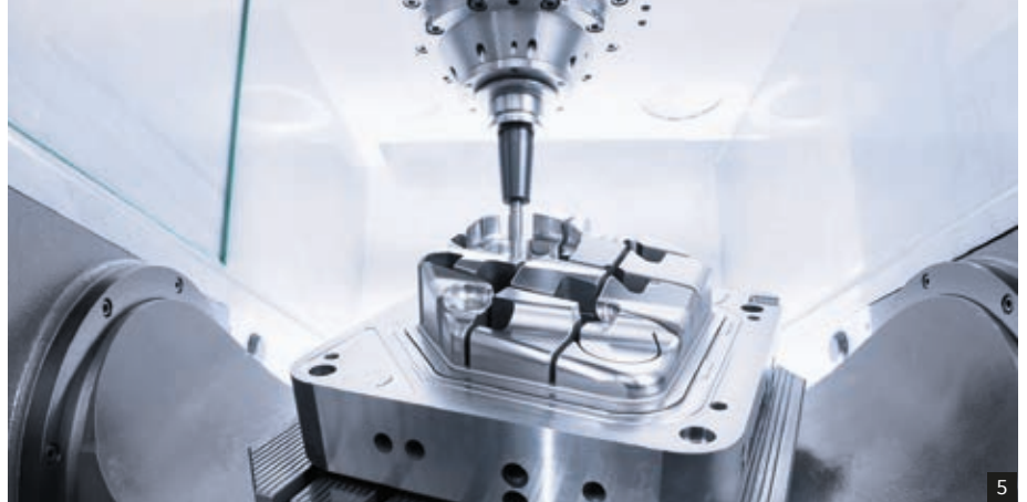
1: Thermosymmetrical gantry design with a gantry drive 2: Tool magazine with a double gripper 3: 5-axis simultaneous machining of an injection mould made from hardened steel 4: Linear drives in X / Y / Z with > 2 g 5: 5-axis machining: integrated NC-swivelling rotary table with torque drives
