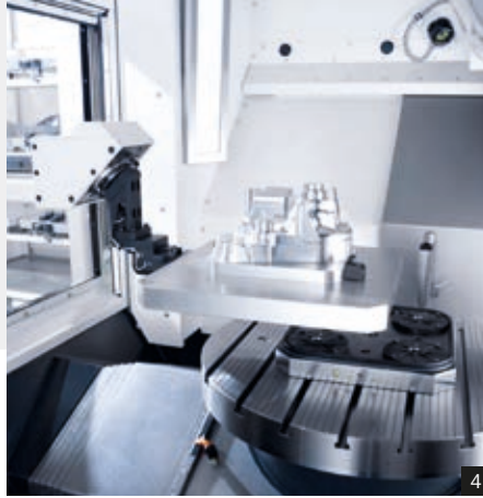
3: Pallet storage for 20 workpieces 4: Pallet handling for parts up to 200 kg
