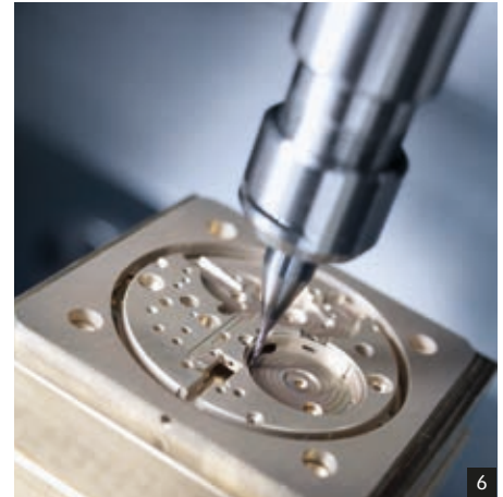
1: Workspace – integrated NC swivelling rotary table 2: 5-axis complete machining of a bone plate in titanium 3: Finish machining of a CoCr femur component 4: Linear drive in X / Y / Z with > 2g 5: 24-pocket tool changer as standard (optional: 60 pockets) 6: Watch mechanism plate
