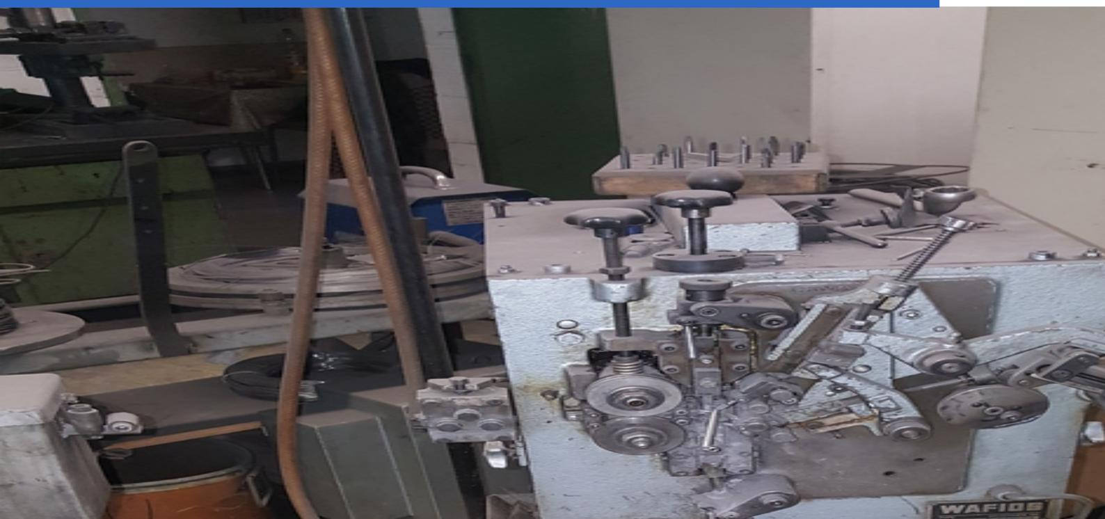
A large industrial coil winding machine, specifically a WAFIOS UFM8 model, is shown in an industrial setting. The machine features a complex assembly of metal components, including a central gear system, various knobs, and a large cylindrical component. Two thick, flexible hoses, one orange and one black, are connected to the machine. The background shows a green wall and some shelving.
