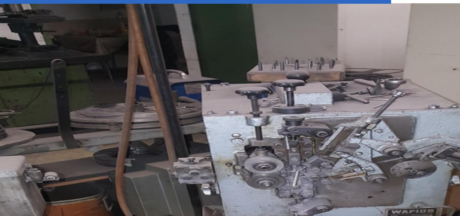
The image shows a large industrial coil winding machine, specifically a WAFIOS UFM8 model. The machine is a complex assembly of metal components, including a central vertical axis with various gears and a horizontal worktable. Two thick, flexible hoses, one orange and one black, are connected to the machine. The background shows a workshop environment with other equipment and green walls.
